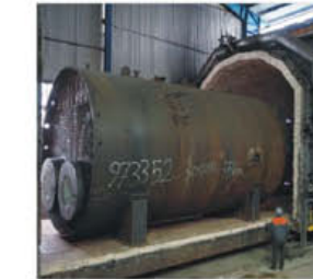
Post-Weld Heat Treatment furnace 1100 °C with a volume of 500 m 3 and temperature accuracy of +/-5 °C
