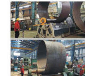
Rolling Machine with 4 hydraulic rollers 3300 mm working width and 60 mm working thickness
