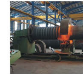
Corrugating Machine 6000 mm length and 25 mm working thickness
