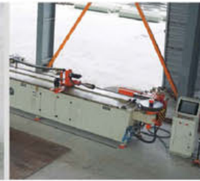
CNC Bend Tube Machine in order to bend tubes from 3/4 inch to 3 inch and working length of 12 meter, capable of rotation. European technology Swaging Machine
