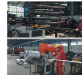
CNC Hydraulic Pipe Rolling Machine capable of working from 3/4 inch to 6 inch
