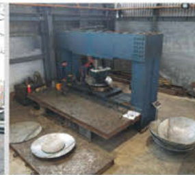
Elliptical Flanging Machine with a working diameter of 4000 mm and a working thickness of 30 mm
