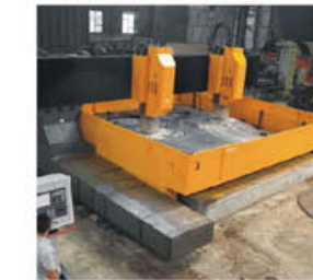
CNC Milling Drill Siemens technology and two spindles (3200 rpm)
