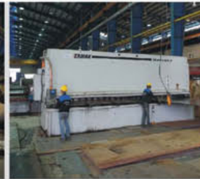
CNC Guillotine Cutting Machine width 6 meters & CNC Brake Press - 300 Ton
