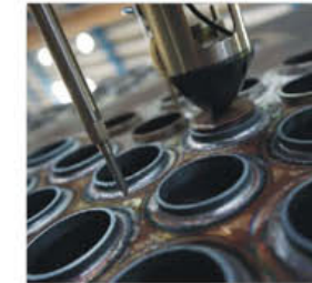
Fully Automatic Orbital Welding Machine of French polysoude brand
