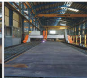
Axis Plasma Cutting Machine with Hypertherm technology of US working width 4300 mm x 15000 mm
